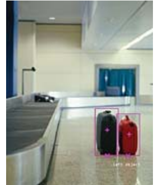
Baggage left unattended in a moving scene can be flagged by intelligent video surveillance systems. Photo courtesy of ObjectVideo
