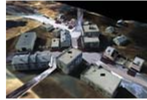
Innovative video technology replaces multiple monitors with a single one that shows a three-dimensional virtual map of a site that the operator uses to access actual views from multiple cameras. Photo courtesy of Pyramid Vision
